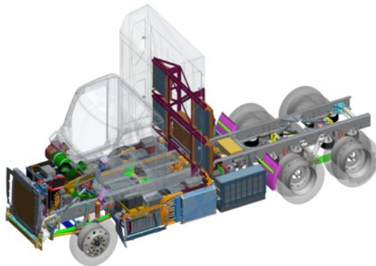
Fuel cell truck packaging layout
